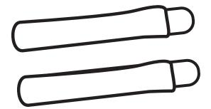
Place a piece of copper wire so that it overlaps about two centimeters from the top of each covered popsicle stick and tape it securely in place covering the exposed wire, like this:
